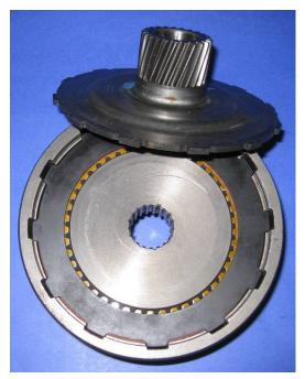
Install the stack-up into the front clutch drum, starting with a steel plate and ending with a friction plate
