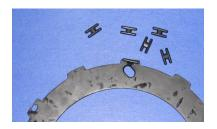
Stack clutch pack on bench; start with a steel plate, make sure the rubber inserts are not stuck under the friction plates and that you do not place lugs that contain rubber inserts on top of each other
