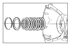
Apply air (40 PSI max) to center support port for the intermediate several times to seat the clutch pack elements. Clutch pack clearance is .040" to .107" (1.02 to 2.72mm) check with feeler gauge between the bottom of the snap ring and the top of the pressure plate.
