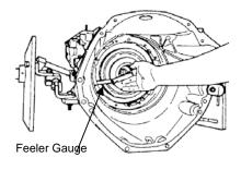
The overdrive clutch pack clearance should be set at .022" to .047" (0.55mm – 1.20mm). Measure using a feeler gauge between the top pressure plate and the selective snap ring. To achieve the recommended clearance, use one of the selective snap rings available from Ford dealer.
