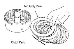
Note: Presoak all friction plates in manufacturer's recommended ATF for 15-20 minutes prior to assembling the clutch pack.
