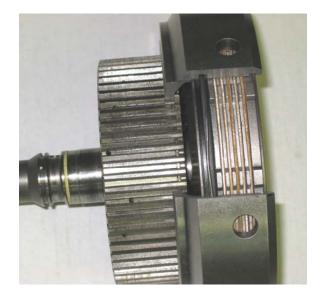
Using air (40 PSI) apply the rear clutch several times to seat all of the clutch pack elements. With a feeler gauge, measure between the bottom of the selective snap ring and the top of the pressure plate. Clearance should be .025" to .050" (0.64 to 1.27mm). Clearance should be correct with the .106" (2.69mm) snap ring provided. However, there are selective snap rings available if needed.
