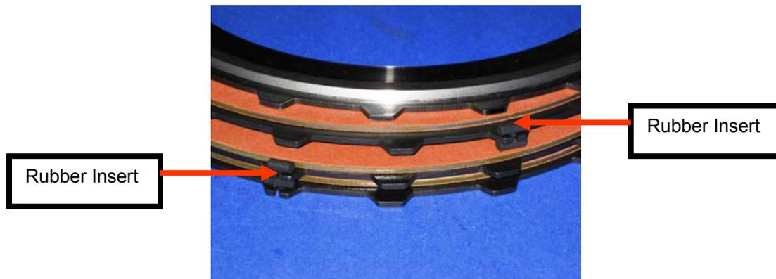
**Caution:** You must install the Kolene® steel plates with rubber inserts in such a manner that the rubber inserts do not stack upon each other, or you will not be capable of completing this stack up.
