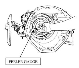
The overdrive clutch pack clearance should be set at .022" - .047" (0.55mm – 1.20mm). Measure by using a feeler gauge between the top pressure plate and the snap ring.
