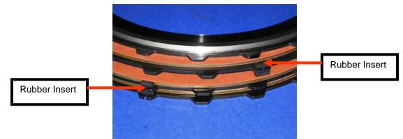
Caution: You must install the Kolene® steel plates with rubber inserts in such a manner that the rubber inserts do not stack upon each other, or you will not be capable of completing this stack up.
