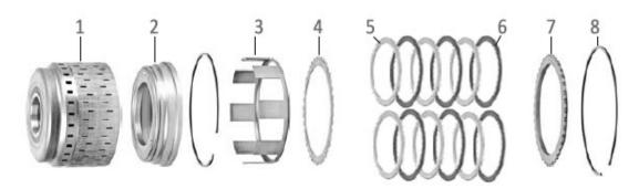
Installation: Stack the Direct clutch pack as follows;
