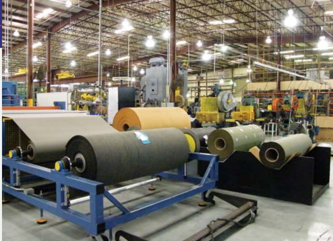
Various rolls of friction papers are easily changed to feed into the die-cutting process that makes the friction-paper component of a clutch. Alto has about eight active formulations for friction characteristics. Variations of those basic formulations result in several dozen different papers being used.
