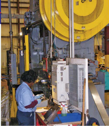
One of a number of stamping machines used to cut out metal discs for clutch-pack steels or frictions and for forming metal bands.
