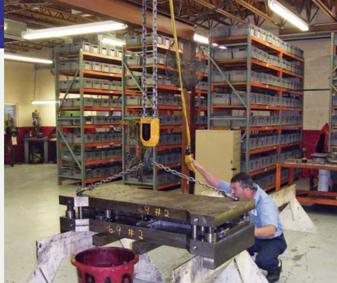
Alto tools and dies for production lines are made and maintained in-house. Here one of the large stamping dies is undergoing periodic maintenance.
