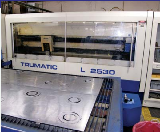
Laser technology is used to cut discs for limited production runs while the high-volume, massive stamping machines are used for high-volume runs.
