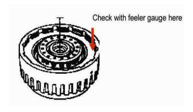
Check clutch pack clearance from the top of the friction disc to the bottom of the pressure plate ledge, using a feeler gauge. Clearance should be .040" - .055" (1.02mm – 1.40mm).
