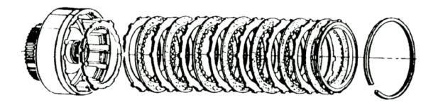
Place the direct clutch onto the center support and apply the clutch several times using air pressure. This will seat the friction and steel elements for a more accurate piston travel measurement. Piston travel specifications are .121" to .236" (3.07 to 6.00mm).
