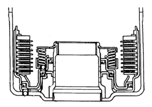
TH 200-4R Stack-up is the same as OE, starting with the .078" Kolene® Steel Plate and the alternately install friction and steel plates ending with the pressure plate. Install the top pressure plate with the micro-finish facing the top friction plate. Clutch pack clearance should be .008" to .010" per lined plate. Check clearance using a feeler gauge between the snap ring and the top pressure plate.
