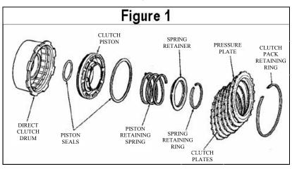
After assembly of drum, apply the clutch pack several times with air to seat all components. See Figure 2.
