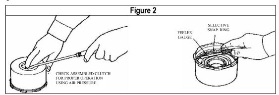
Check clutch pack clearance using a feeler gauge. Insert feeler gauge between selective snap ring and pressure plate. Adjust clearance to .025" - .050" (0.6mm – 1.27mm).
