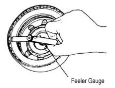
Apply air to assembled clutch pack several times to seat the friction and steel elements. Use a feeler gauge to measure between the bottom of the selective snap ring and the top of the pressure plate. Clearance should be .040" to .075" (1.02 to 1.91mm). To achieve the recommended clearance, use one of the selective snap rings available from Alto Products Corp.
