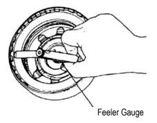
Apply air to assembled clutch pack several times to seat the friction and steel elements. Using a feeler gauge measure between the bottom of the selective snap ring and the top of the pressure plate. Clearance should be .040" to .075" (1.02 to 1.91mm). Adjust clutch pack clearance by selecting the correct selective snap ring.
