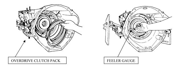
The overdrive clutch pack clearance should be set at  $.022^{\circ}$  -  $.047^{\circ}$  (0.55mm – 1.20mm). Measure by using a feeler gauge between the top pressure plate and the snap ring.
