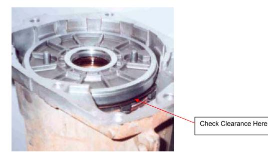
Before installing the wire snap ring, measure the clearance between the top steel plate and the apply piston with a feeler gauge or drill bit. Clearance should be .095" to .115" (2.41 to 2.92mm). Clearance can be adjusted with one of ten selective shims which are available through Chrysler. Once the clearance is correct, install the wire snap ring.
