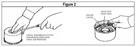
Check clutch pack clearance using a feeler gauge. Insert feeler gauge between selective snap ring and pressure plate. Adjust clearance to .025" - .050" (0.6mm – 1.27mm).
