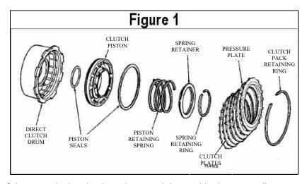
After assembly of drum, apply the clutch pack several times with air to seat all components. See Figure 2.
