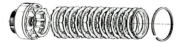
Place the direct clutch onto the center support and apply the clutch several times using air pressure. This will seat the friction and steel elements for a more accurate piston travel measurement. Piston travel specifications are .121" to .236" (3.07 to 6.00mm). Clutch pack clearance should measure between .060" to .080" using feeler gauges.
