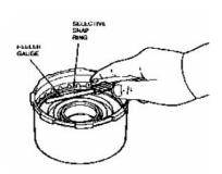
Check clutch pack clearance using a feeler gauge, insert feeler gauge between selective snap ring and pressure plate. Adjust clearance to .025" - .050" (0.6mm - 1.27mm).
