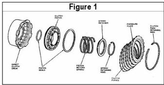
After assembly of drum, apply the clutch pack several times with air to seat all components, see Figure 2.
