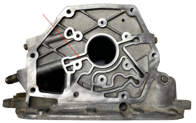
3. Continue installing retainer using recommended OE procedures, do not force the retainer into the case, because of case machining differences, you may have to slightly hone the case to achieve proper alignment and fitment.
