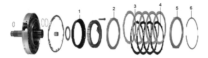
**Installation:** Stack the Overdrive clutch pack as follows; install modified apply piston (1), install return spring and retaining bolts, install the bottom .192" apply plate (2), install a friction (3), install a Kolene® steel plate (4), You will be alternating friction and steel plates, 5 frictions and 4 steel plates, install top .192" pressure plate (5) and original snap ring (6)
