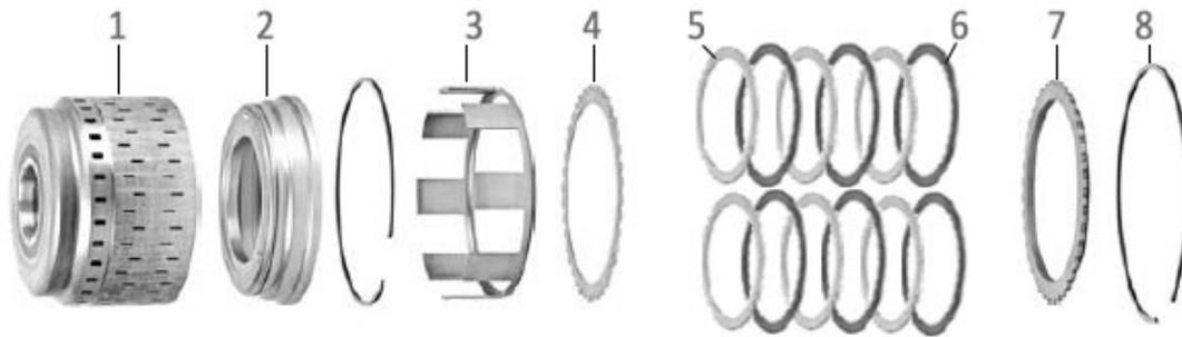
**Installation:** Stack the Direct clutch pack as follows;
