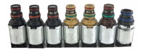
GM 6T40, 6T45 (Gen 2) OEM 7 Piece Solenoid Kit 2012-On
