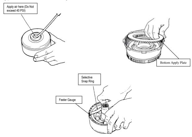
Apply air to assembled clutch pack to seat friction and steel elements. Check clutch pack clearance using a feeler gauge, measure between the top of the pressure plate and the bottom of the selective snap ring. Clearance should be .040" to .075" (1.02 to 1.91mm) Clutch pack clearance can be adjusted by one of four selective snap rings available from Alto Products..
