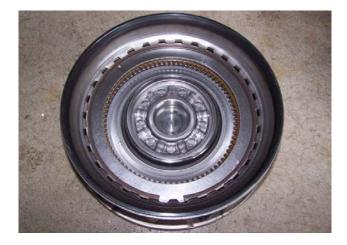
**215758B (OE 2 friction plate)** Prepare the externally splined steel plates by installing inserts into the teeth.
